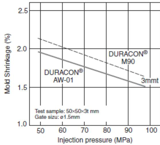
**Fig. 2-4 Mold Shrinkage**
