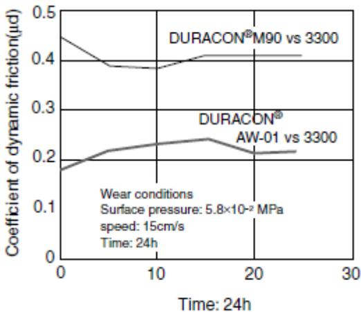
Fig. 1-6 Coefficient of Dynamic Friction against DURANEX® PBT 3300
