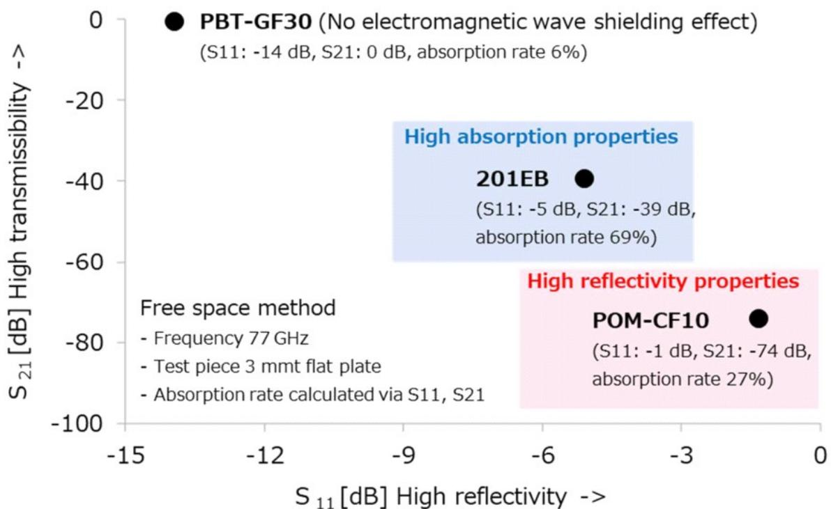
Figure 2-1: DURANEX® PBT 201EB millimeter wave transmissibility, reflectivity, and absorption rate
