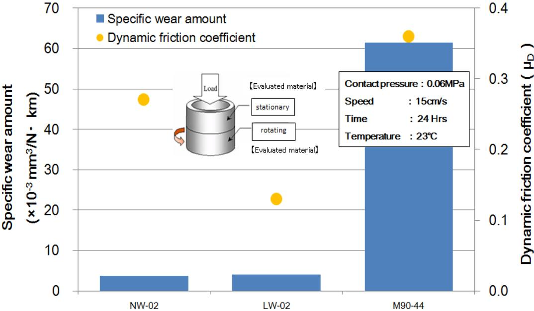
Figure 2-1 Comparison of friction and wear characteristics (when both mating materials are the same)
