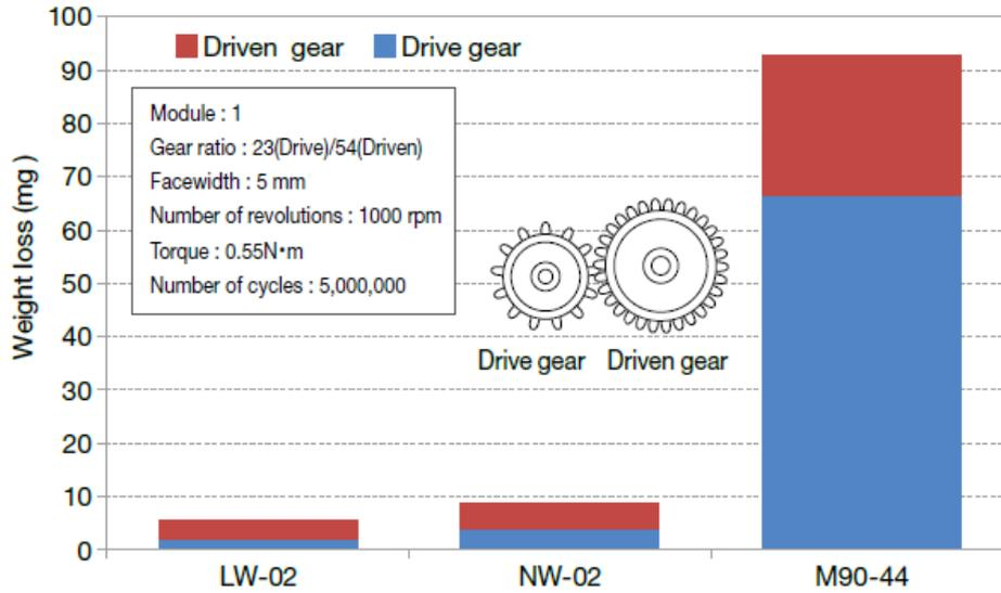
Figure 3-3 Gear wear (against the same material)
