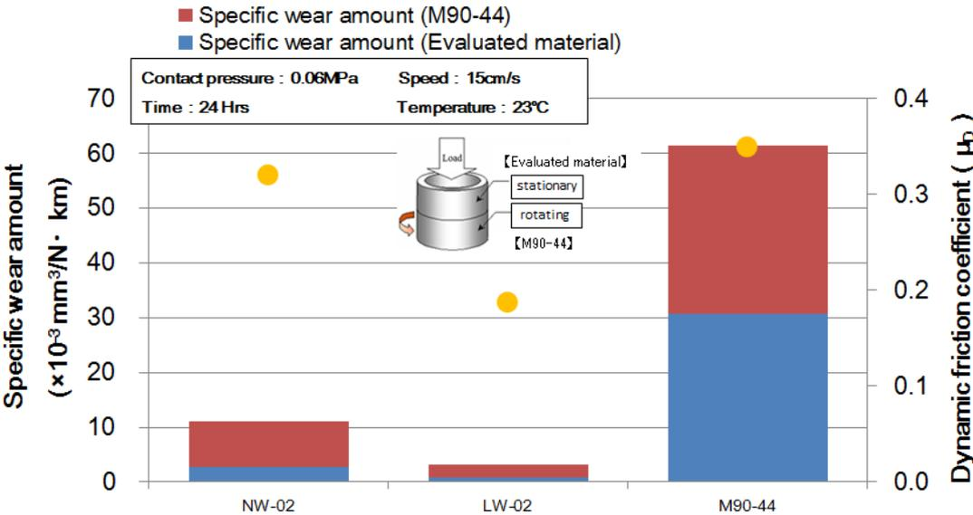
Figure 2-2 Comparison of friction and wear characteristics (when mating material is M90-44)
