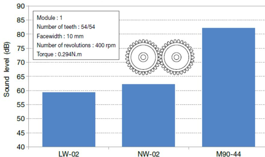
Figure 3-2 Gear noise (against the same material)
