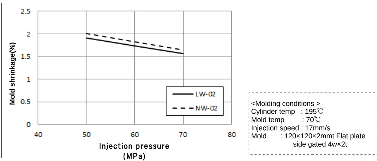
Figure 4-2 Mold shrinkage (2mmt)
