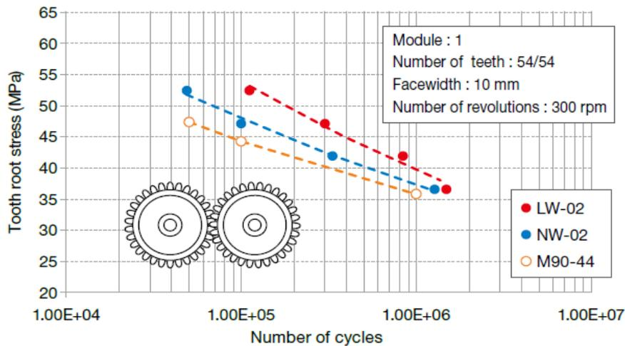
Figure 3-1 Gear tooth surface fatigue (against the same material)
