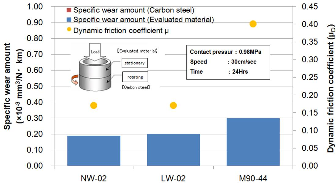
Figure 2-3 Comparison of friction and wear characteristics (when mating material is Carbon Steel)
