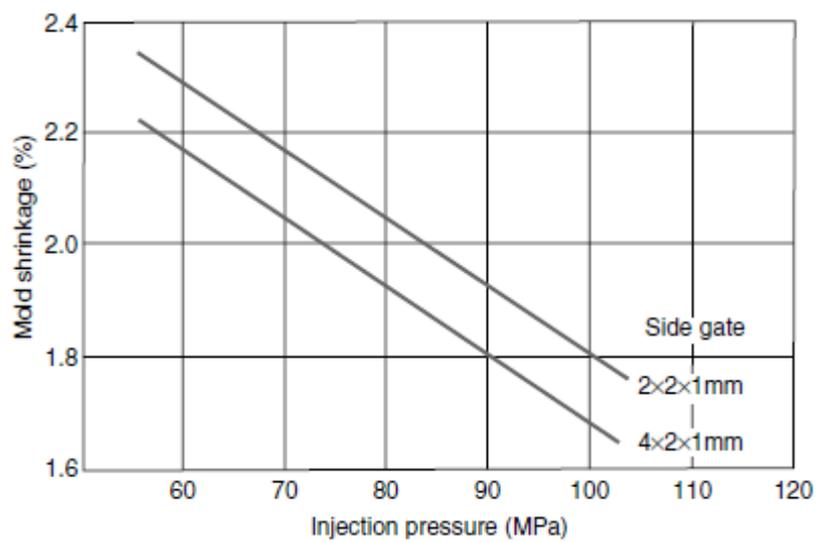
**Fig. 3-8 DURACON® POMM270-44 mold shrinkage ratio**
