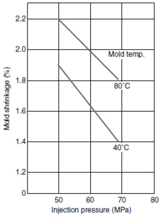
**Fig. 2-11 DURACON® POM M450-44 mold shrinkage ratio (3mmt)**
